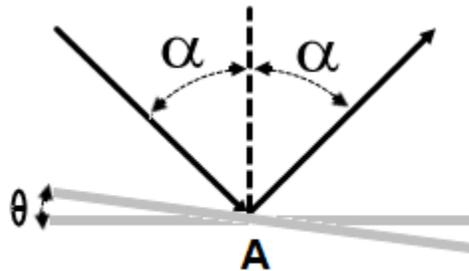
3. A narrow beam of light is incident on the surface of a plane mirror. The initial angle between the incident ray and reflected ray is  $2\alpha$ . If the mirror is turned around point A by the angle  $\theta$  what is the change of the angle between two rays?
