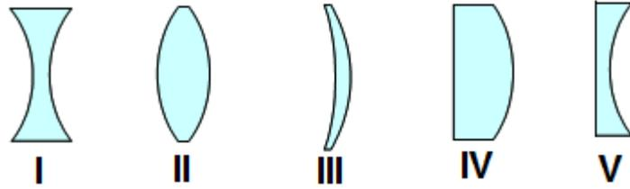
18. Which of the lens or lenses is the converging lens?
