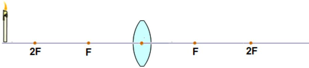
2. An object is placed at a distance of 60 cm from a converging lens with a focal length of 20 cm.
