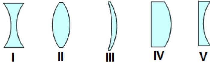
19. Which of the lens or lenses is the diverging lens?
