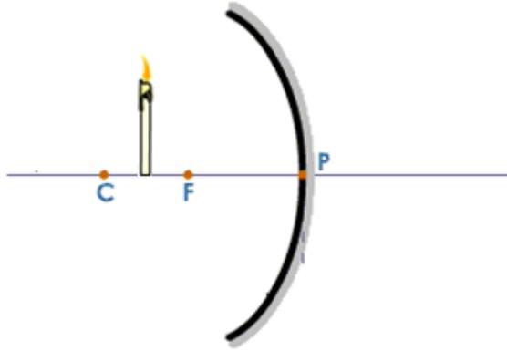
1. A candle is placed at a distance of 15 cm from of a concave mirror with a focal length of 10 cm. The candle is 4 cm tall.
