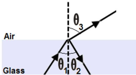
5. A light ray travels from glass to air at an angle of incidence  $\theta_1 = 35^\circ$ . The ray partially reflected from the glass-air boundary at the angle  $\theta_2$  and partially refracted at the angle  $\theta_3$ . The index of refraction of the glass is 1.6.
