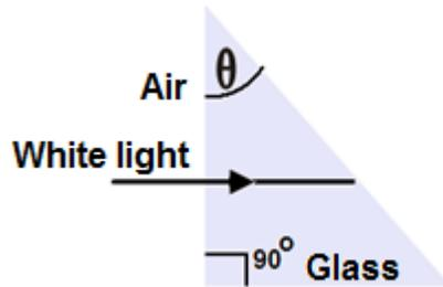
6. A narrow beam of white light is incident normally on the surface of a triangular silicate flint glass prism with one angle of  $90^\circ$ . The index of refraction for violet light is 1.66 and for red light is 1.61. The angle  $\theta$  in the prism is less than the critical angle for this type of glass.
