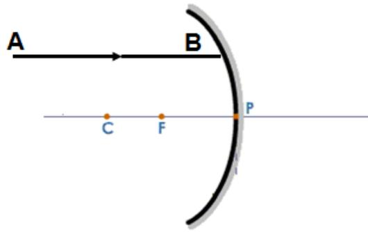
8. A very narrow light ray AB strikes the surface of a concave mirror as shown on the diagram. Which of the following diagrams represents the reflected ray?
